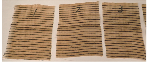
Photo 2 Soaking test of brown pieces of used Bashofu.
