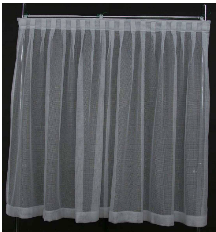
Fig.3-2 An example of curtains (Interval of pinched parts:5cm)
