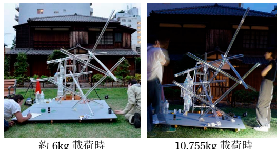
Fig.9 Vertical loading of the mockup
