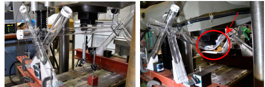
Fig.7 Experiment with the frame and connections (left: before loading, right: after fracture)
