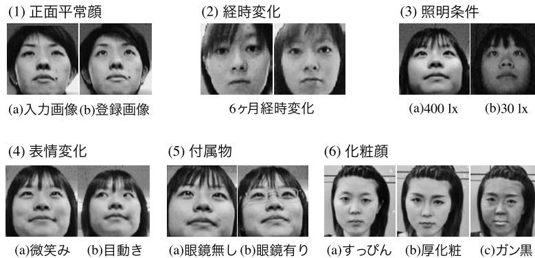
Fig. 1 Samples of recognizable facial images in a conventional system with front images database.
